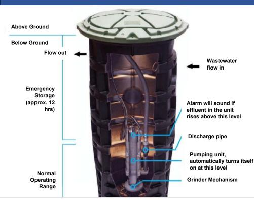
The system consists of a pumping unit which is connected to a network of pipes from other properties in vour area.
