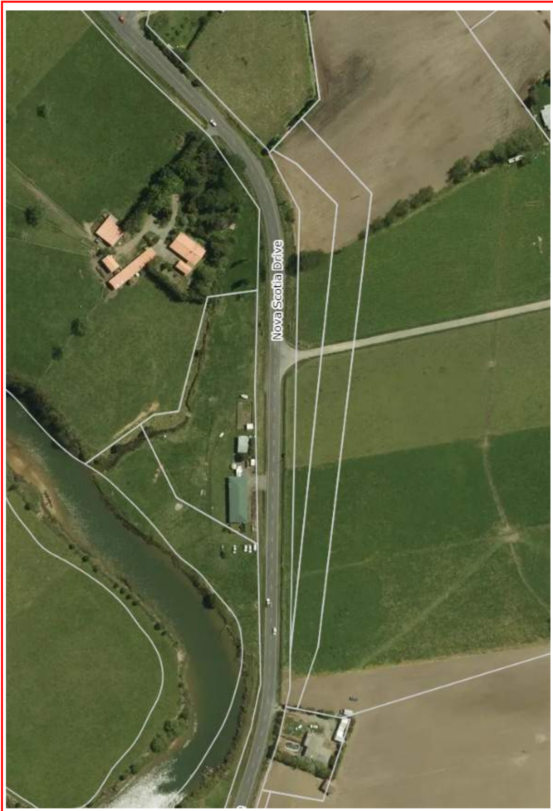
Figure 13: Road reserve boundaries on Nova Scotia Drive
