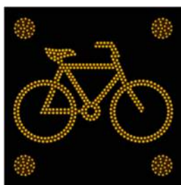
Figure 31: W19-2.1 Symbolic Warning – Active LED (Cyclist symbol as in W16-7)
