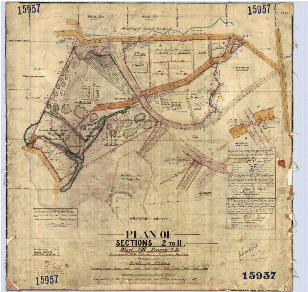
Figure 7: Detail from SO 15957 (1910) showing tramway, incline, ballast pit, railway water pipe and other features of interest.
