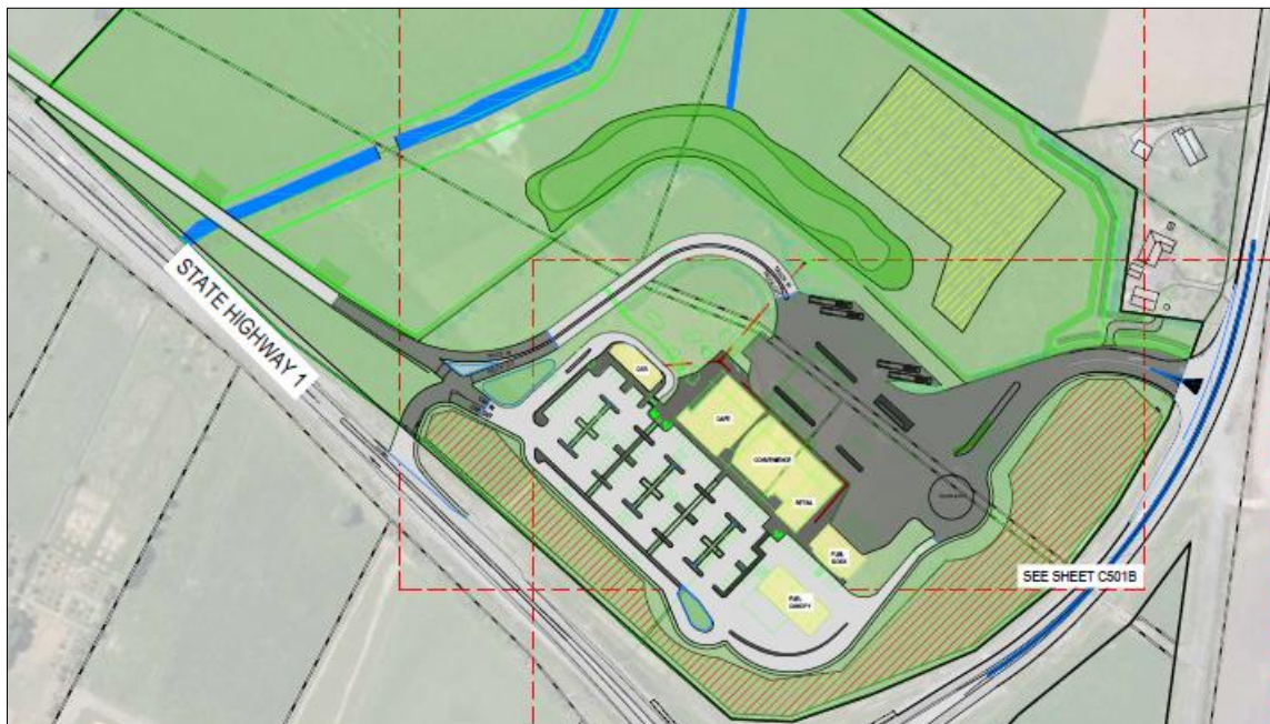
Figure 11B: Wastewater treatment system and disposal fields
