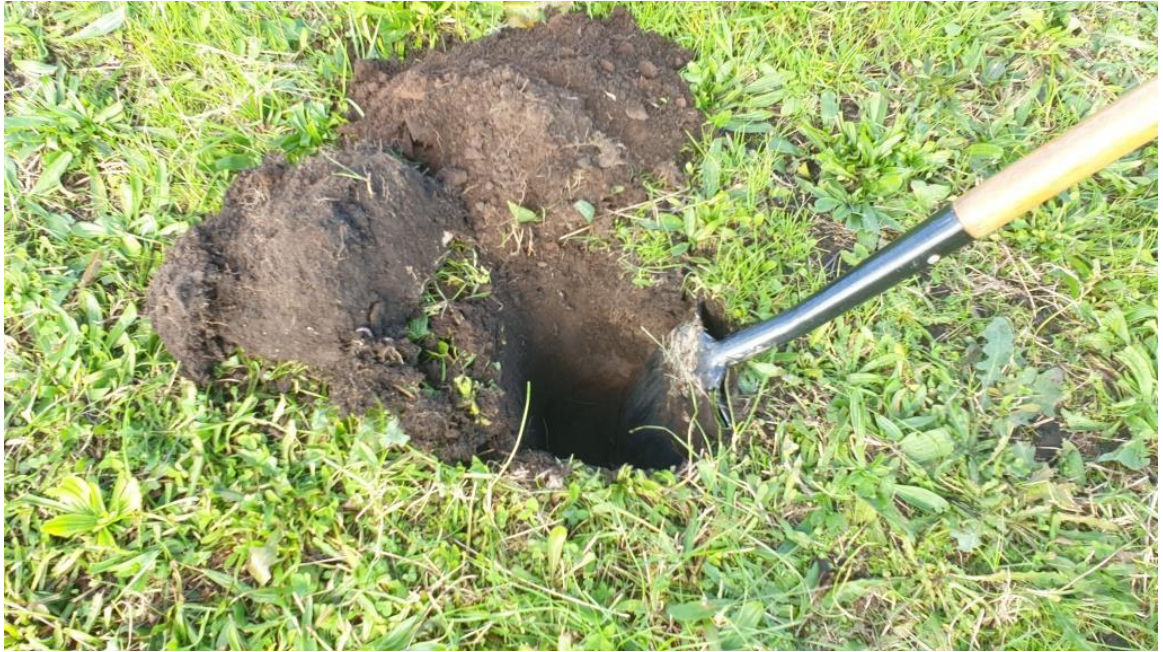
Figure 30. Dry peat soils exposed in Test Pit 1 at the eastern boundary of the property
