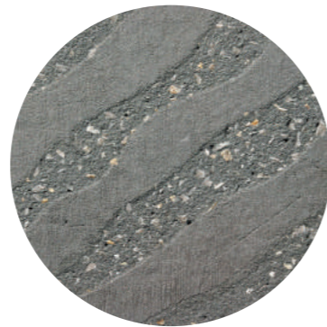
Sandblast Exposed Aggregate
