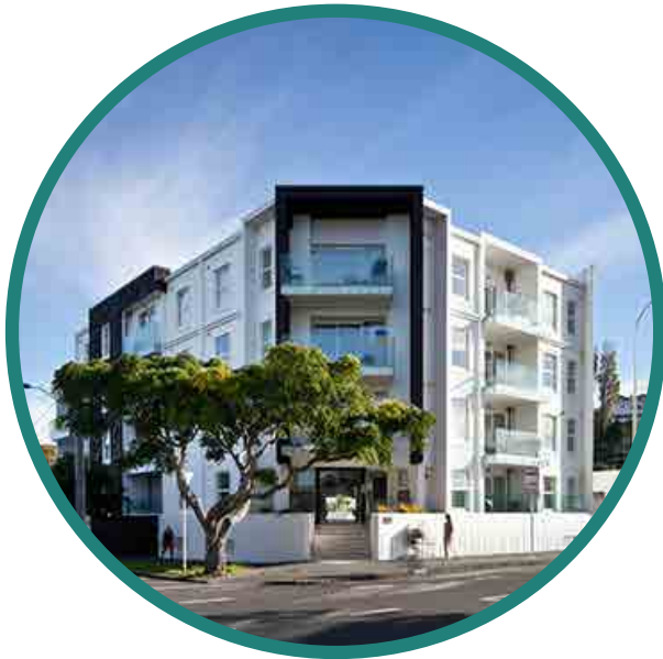
Guideline 5 This corner apartment addresses both adjacent streets as well as containing a prominent entranceway at the apex.
