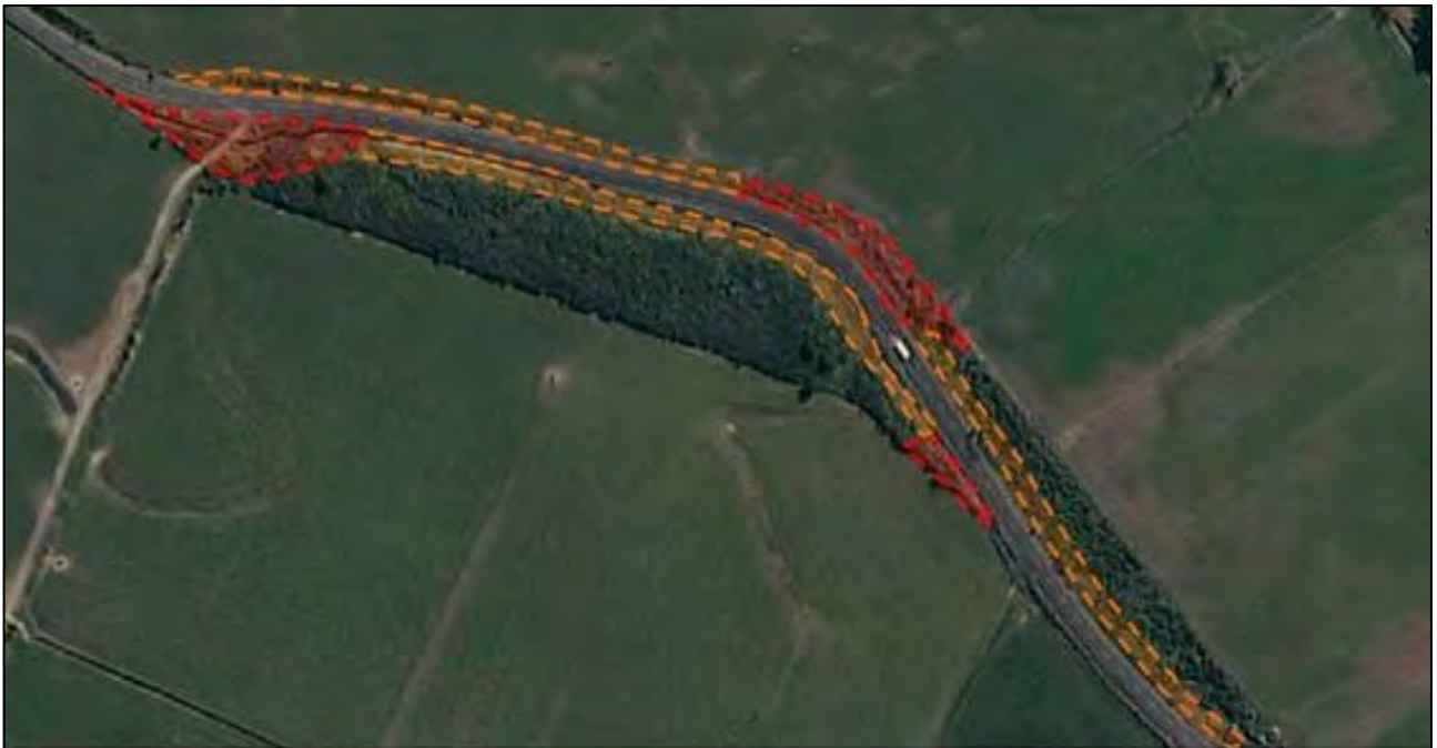
Diagram 4: Location of planting limitation zones; the red areas are tree exclusion ‘vehicle runoff’ zones (no trees to be planted >100mm diameter), and the orange indicate a 1.5 – 2 metre planting exclusion set back for road maintenance (no planning whatsoever) (source WDC)
